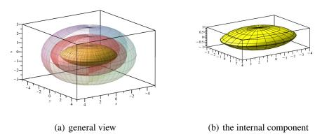
Figure 12: Envelope of unit spheres center on an ellipsoid - (a, b, c) = (4, 4, 2)
